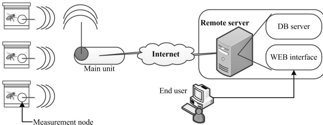
Fig. 6. Wireless measurement system used in ITAPIC project.
